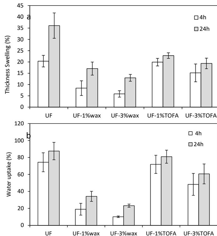
Figure 3. Thickness swelling (a) and water uptake (b) of MDF categories manufactured by using bio- or petroleum-based additives (TOFA, wax). The bars show standard deviation.
