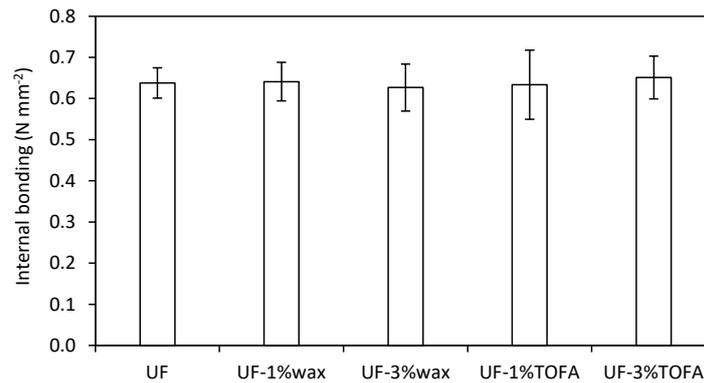
Figure 2. Mean internal bonding (IB) of MDF categories manufactured by using bio- or petroleum-based additives (TOFA, wax). The bars show standard deviation.
