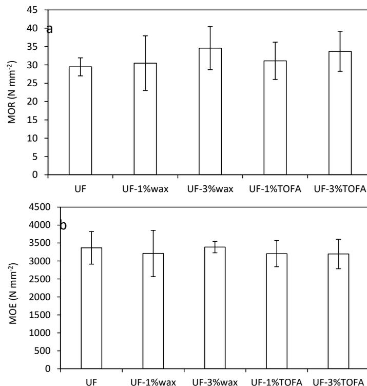
*Figure 1. Mean moduli of rupture (MOR, a) and elasticity (MOE, b) of MDF categories manufactured by using bio- or petroleum-based additives (TOFA and wax). The bars show standard deviation.*
