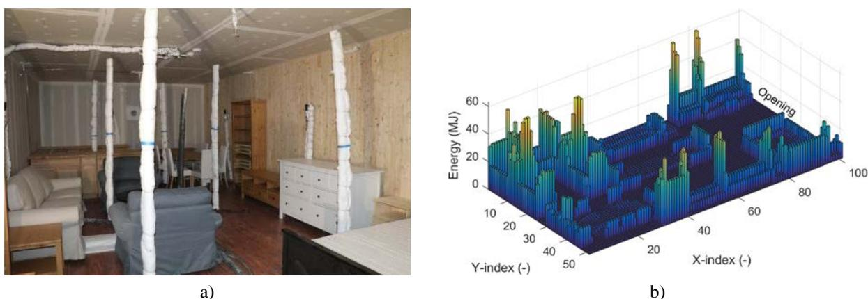
Fig. 2. a) Photograph of movable fuel as installed; b) Model of fuel energy distribution in the compartment
