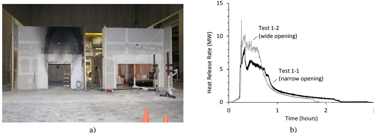
Fig. 4. Influence of opening size on the measured heat release rate for the same movable fuel load of  $550 \text{ MJ/m}^2$  and no participation of CLT: a) Test 1-1 with narrow opening; b) Test 1-2 with wide opening
