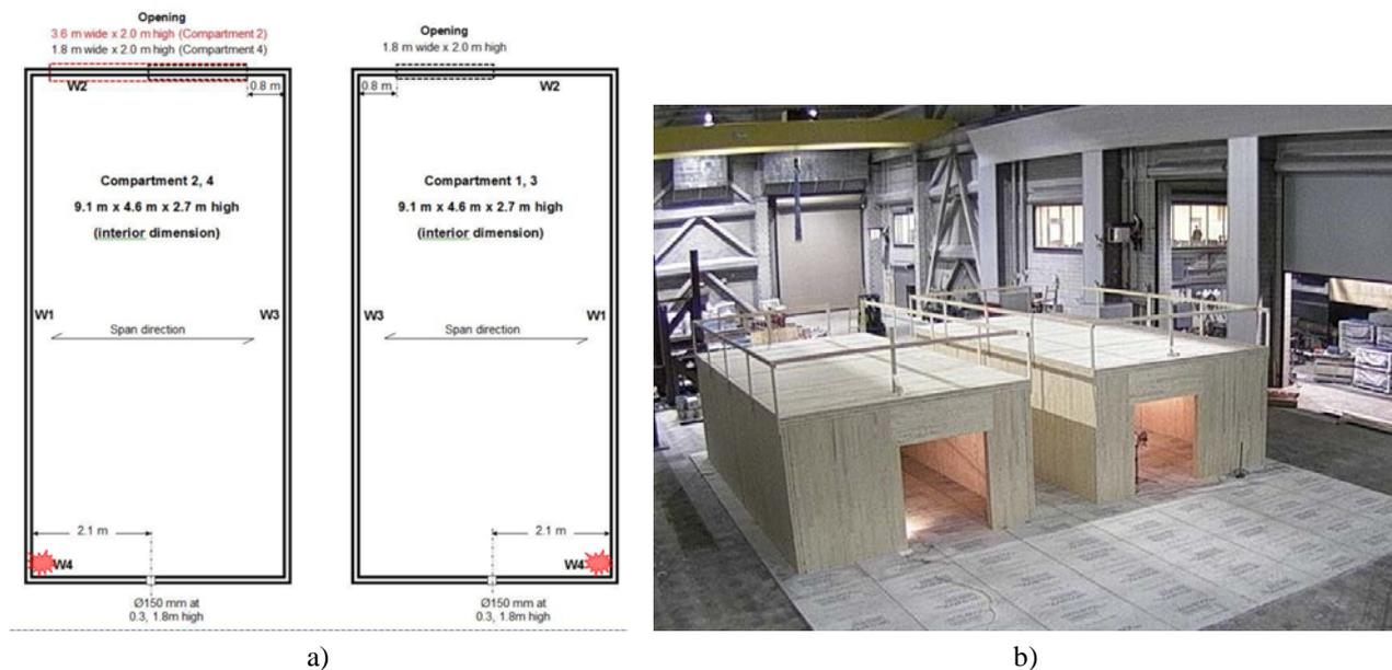
*Fig. 1.* a) Plan view schematic of test compartments; b) Photograph of test compartments (bare structure)
