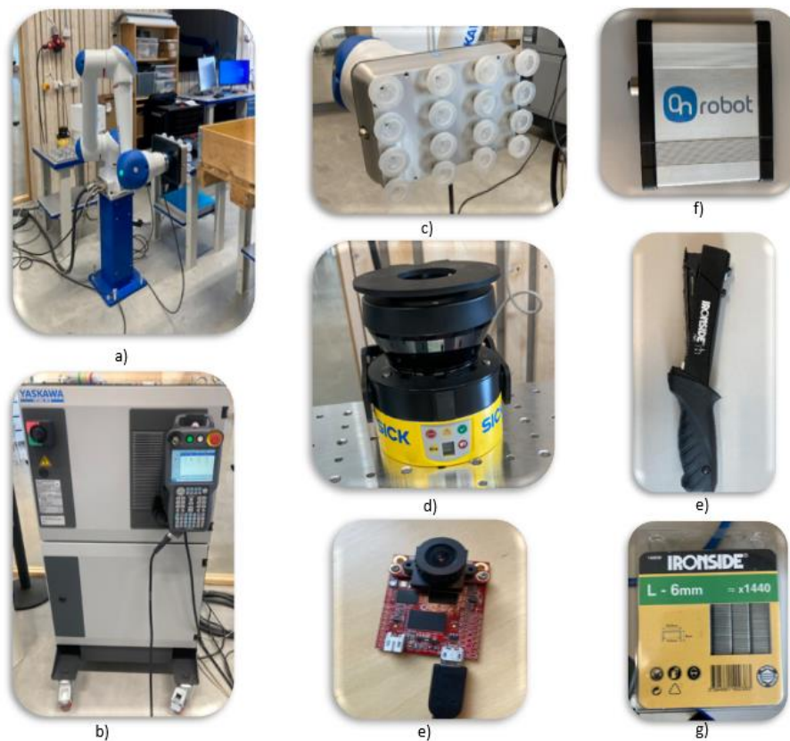
Figure 5.1: Shows all the equipment used in the set-up a) Yaskawa HC10 b) YRC1000 HC10 c) VGP20 d) SICK S300 Mini e)OpenMV h7 plus R3 f)ComputeBox e)Hammer Tacker g)Staples
