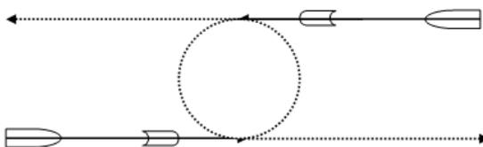
**Fig. 4 180° simultaneous turn**
