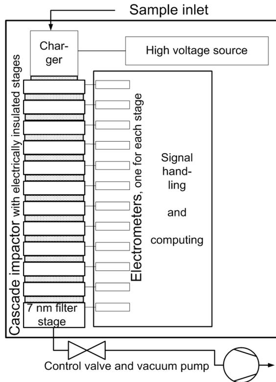
Fig. 3-3: Principle of the Electric Low Pressure Impactor, ELPI
