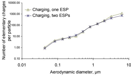
Fig. 4-4: Normalized charge of particles penetrating one and two ESPs respectively
