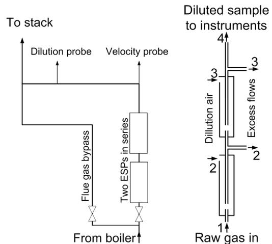
Fig. 3-2: To the left is shown the position of the two tested ESPs in the modified flue gas lines, together with the sampling points. To the right is shown the principle arrangement of the dilution probe.
