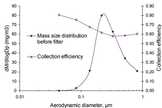
Fig. 4-3: Collection efficiency based on ELPI data for two ESPs in series together with the additional particle trap
