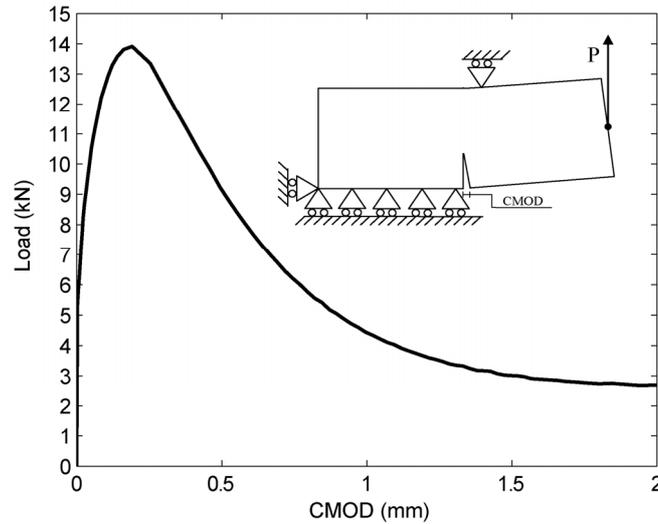
Figure 10. Load in the rail as a function of crack mouth opening displacement, CMOD for the vertical crack. The relation is obtained using the FCM.
