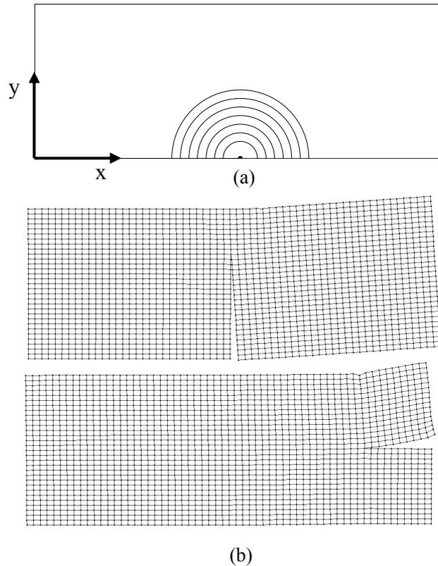
Figure 7. (a) The position of the pith was set to  $(x,y) = (60,0)$  mm. (b) The mesh used in the analyses with cracks that have propagated. Deformations are magnified 10 times.
