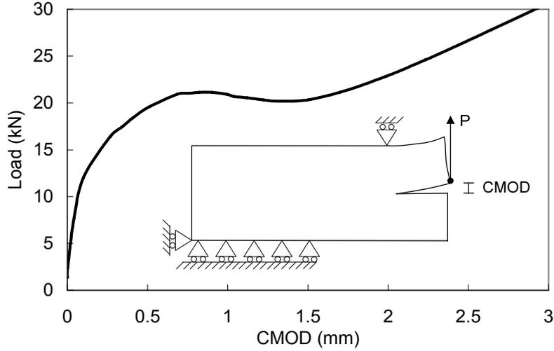
Figure 12. Load in the rail as a function of crack mouth opening displacement, CMOD for the horizontal crack. The relation is obtained using the FCM.
