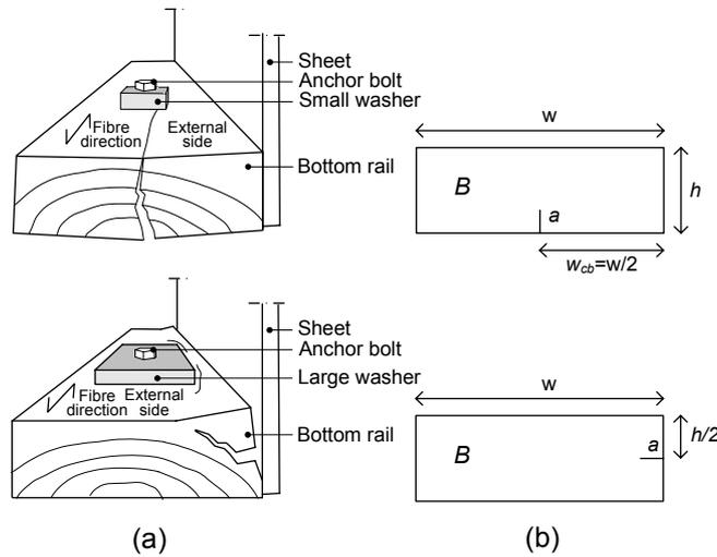
Figure 1. (a) Bottom rail at failure due to splitting. The rail is anchored to the substrate by means of an anchor bolt and a washer. (b) Parameters used in the current study for analyzing the rail.
