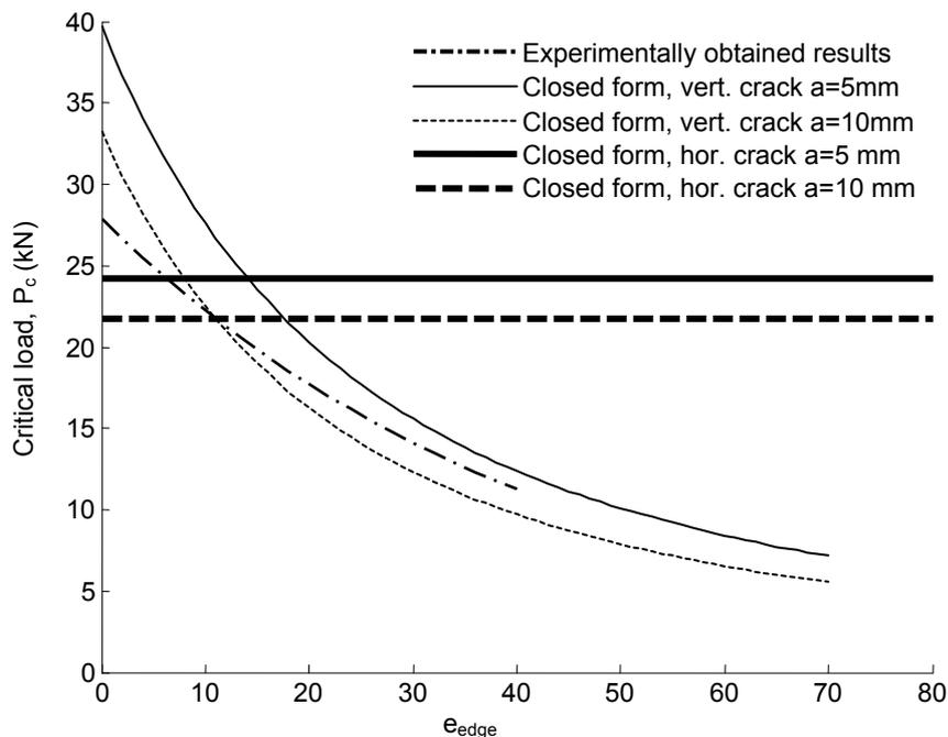
Figure 13. Comparison of results according to an empirical expression based on experiments and according to analytical models (eqs. 6 and 9). The curves show critical load versus length from washer edge to rail edge,  $e_{edge}$ . Washer size is here 40 mm. Horizontal curves correspond to a horizontal crack (eq.9.)
