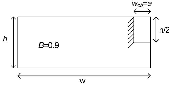
Figure 5. Simplified, one end of the rail may be seen as a cantilever beam with the length,  $w_{cb}$ , being equal to the length of the crack,  $a$ , and the height  $h/2$ .
