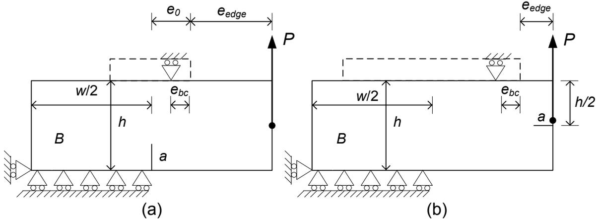
Figure 6. Geometry and applied load case for the studied rail with (a) a vertical crack and (b) a horizontal crack, each with the length  $a$ . The position of the washer (substituted by a boundary condition in the analyses) is indicated with dashed lines.
