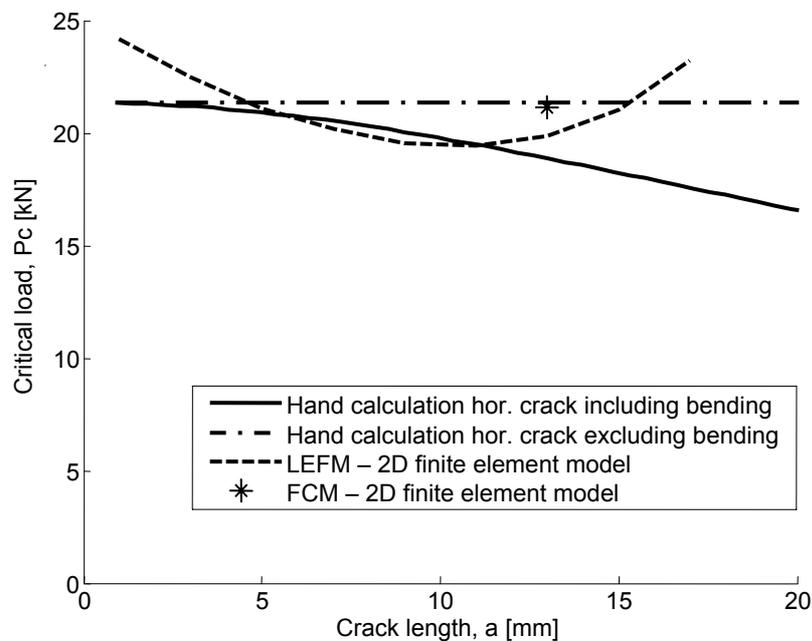
Figure 11. Critical load,  $P_c$ , as a function of crack length according to the closed form expression (solid line) and the LEFM FE simulation (dashed), both for the horizontal crack. The asterisk indicates the critical load according to the FCM analysis, which appears at a state corresponding to a crack length of about 13 mm.
