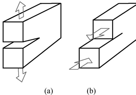
Figure 3. Mode I (a) and mode II (b) loading.
