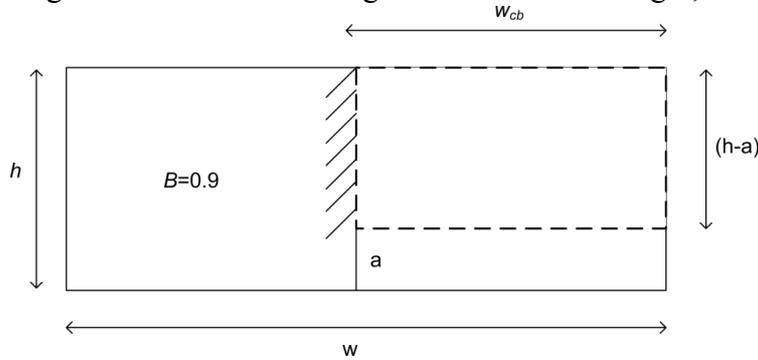
Figure 4. One end of the rail is considered a cantilever beam with the length  $w_{cb}$  and the height  $(h-a)$ .
