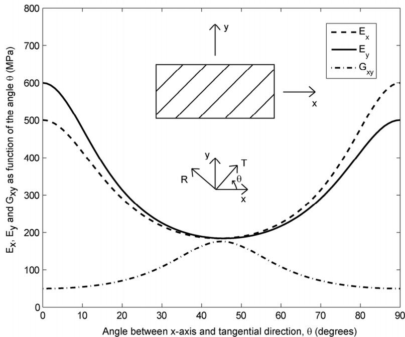
Figure 2. Influence of annual ring orientation on the effective moduli of elasticity and shear modulus referring to the global x-y-coordinate system.
