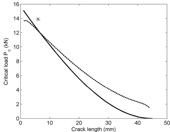
Figure 9. Critical load,  $P_c$ , as a function of crack length according to the closed form expression (solid line) and the LEFM FE simulation (dashed), both for the vertical crack. The asterisk indicates the critical load according to the FCM analysis, which appears at a state corresponding to a crack length of about 6 mm.
