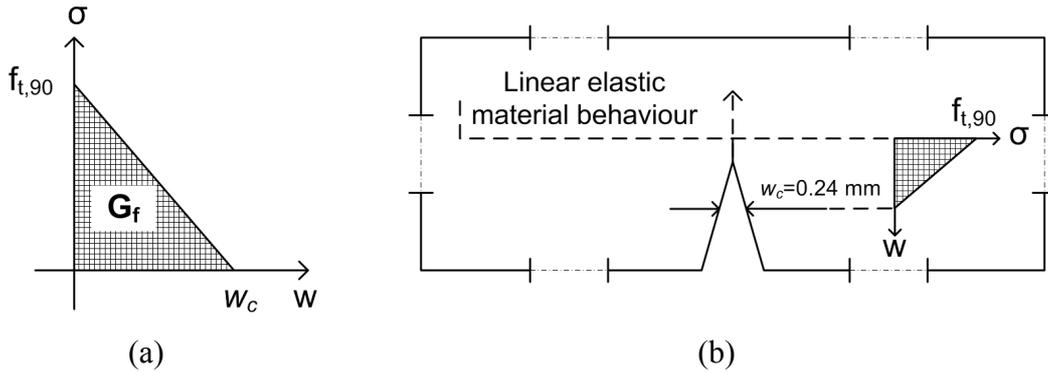
Figure 8. (a) A linear softening behavior was assumed in the FCM, defining the critical opening displacement,  $w_c$ , where no stress can be transmitted. (b) Above the crack, i.e. above the position where the stress level is equal to  $f_{t,90}$ , the material behaves linearly elastically.
