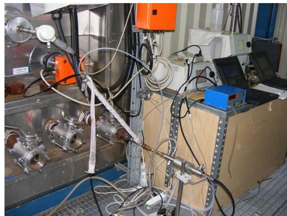
Fig. 4: Ongoing particle size measurement at the ESP outlet.
