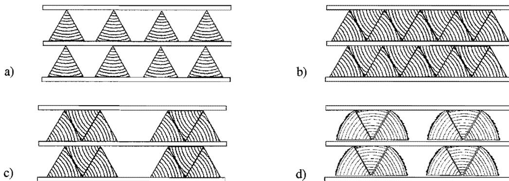
Figure 3. Arrangement of triangular profiles; (a) simple stacking, (b) in blocks, (c) in groups of three, (d) unedged triangles in groups of three.
