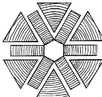
Figure 1. Star-sawing - a new sawing pattern to produce timber with vertical annual rings free from pith and most of the juvenile wood.
