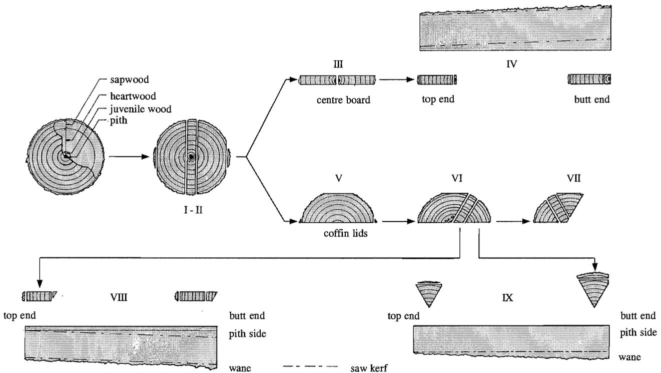
Figure 4. A schematic presentation of star-sawing in practice.
