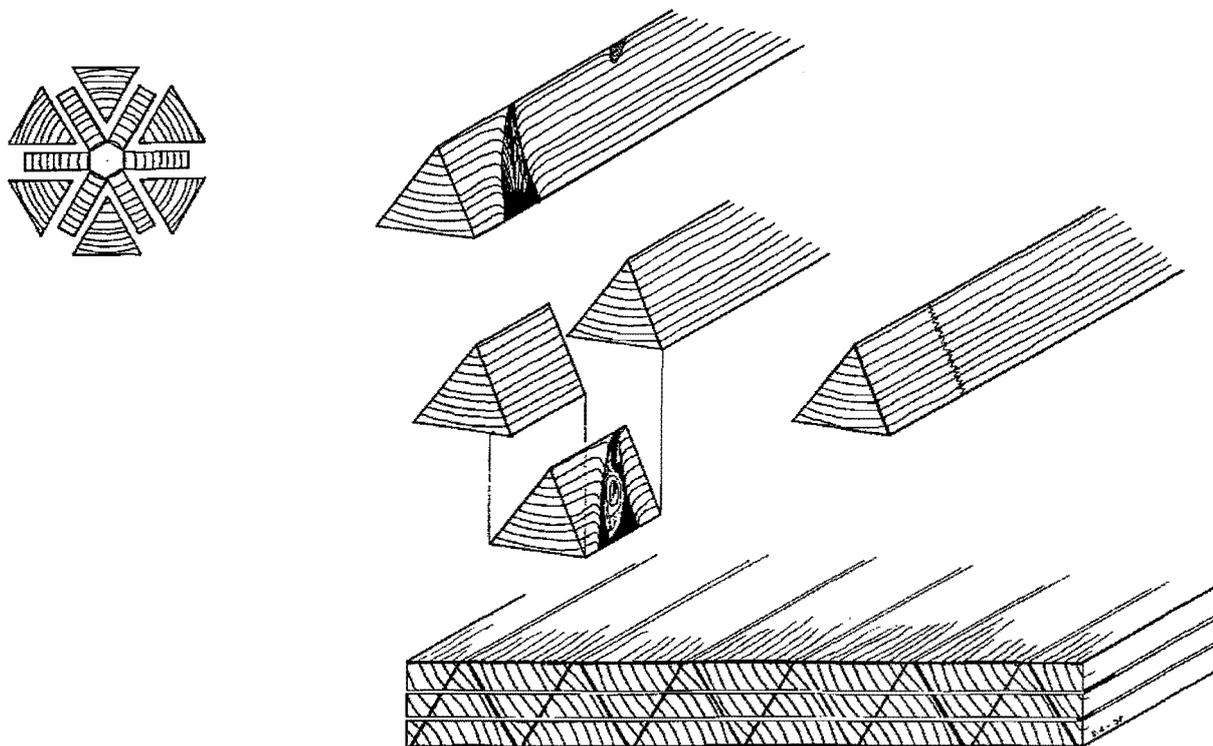
Figure 6. PrimWood Prism, defect-free triangles glued together into a block.
