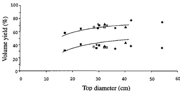
Figure 2. Volume yield with respect to the top cylinder volume for star-sawing from simulations and test sawings between the years 1993 and 1998 [1]. Unbroken curves are estimated volume yield according to Sandberg [2].
