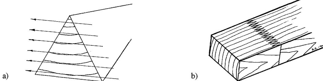
Figure 5. Finger-jointing of the triangles can be carried out in different ways giving a different appearance of the join in the visible surface. Finger cutting parallel to the tangential surface of the triangles (a) gives a zigzag pattern in the surface when the triangles have been glued together (b).
