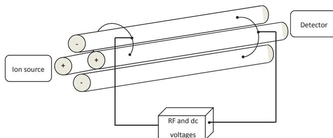
Figure 5. Configuration of a quadrupole mass filter. Adapted from Miller and Denton, 1986 with permission from American Chemical Society.
