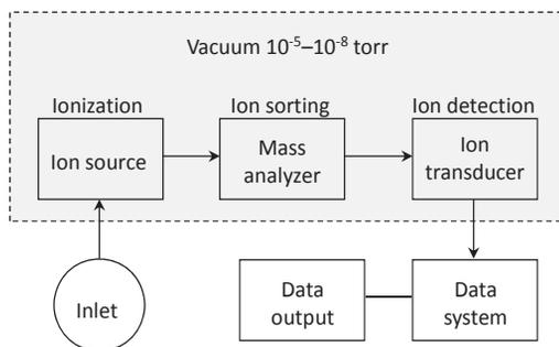
Figure 4. Organization of different units in a MS. The figure is adapted from Skoog *et al.*, 2007 with modifications.
