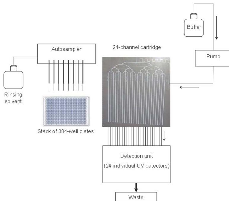
Figure 16. Schematic diagram of the Nanostream platform including a 24-channel cartridge that served as parallel affinity capillaries and a 24-detector unit. The figure is from *paper I* with permission from John Wiley & Sons.
