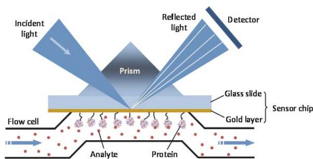
Figure 3. A scheme of the fluidic system in SPR instrumentation. The figure is adapted from *Biacore Handbook* (Biacore, 2008) with permission from GE Healthcare.
