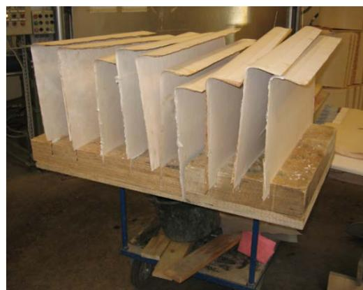
a) *Mould where the shell was laminated, and b) stance for newly pressed shells.*
