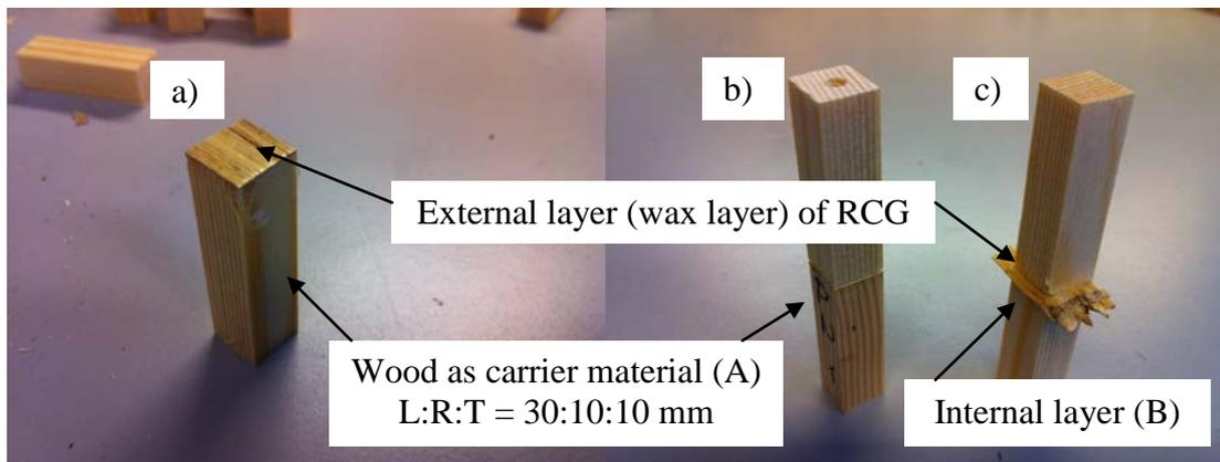
**Fig. 1** Design of the samples. a) Reed canary grass (RCG) glued onto wood with PVAc as its internal layer, and b) and c) in a second step by another adhesive to the test bonding between the adhesive and external layer
