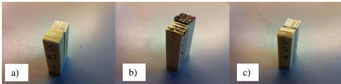
**Fig. 2.** Examples of fracture surfaces of the test specimens: a) wax-layer (uniform), b) wax-layer (irregular), c) both layers (uniform)
