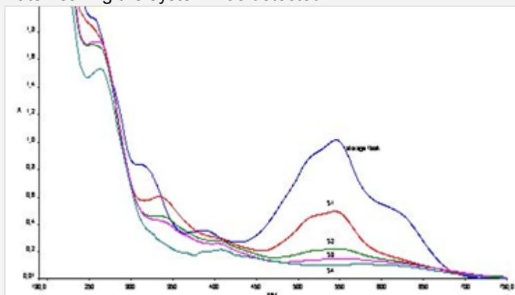
Fig. 1: absorbance curves for original dye mix and after each treatment reservoir at a turnover time of 56.8 h, with 2 gl<sup>-1</sup> at 20°C.
