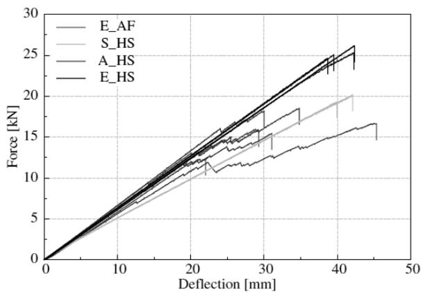
Figure 5: Load-deflection plots of beam tests using different adhesives and glass qualities
