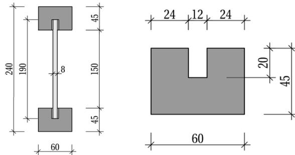
Figure 3: Cross-section of beams
