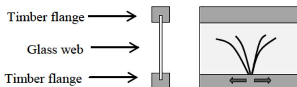
Figure 1: Schematic idea of the concept for timber-glass composite beams: cross-section of the hybrid beam (left), side-view of the beam with cracked glass web (right)
