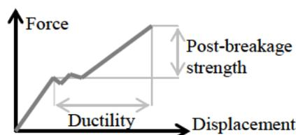
Figure 2: Force-displacement diagram presenting idea of ductility and post-breakage strength of timber-glass composite beams
