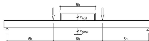
Figure 4: Loading scheme and testing machine
