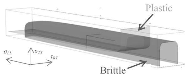
Figure 1 Combination of failure surfaces for plastic and brittle failure modes by super-ellipses
