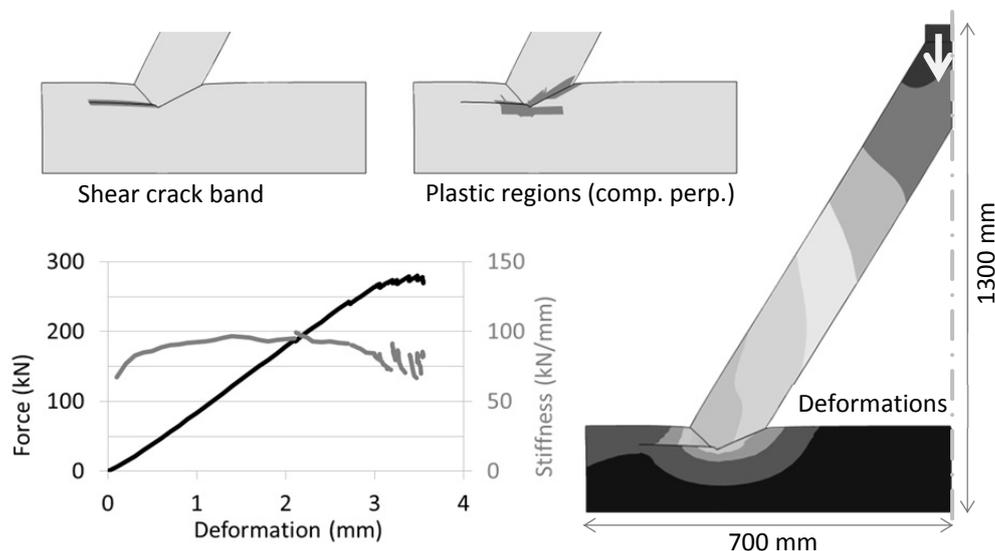
Figure 2 Geometry and results for a woodworking joint
