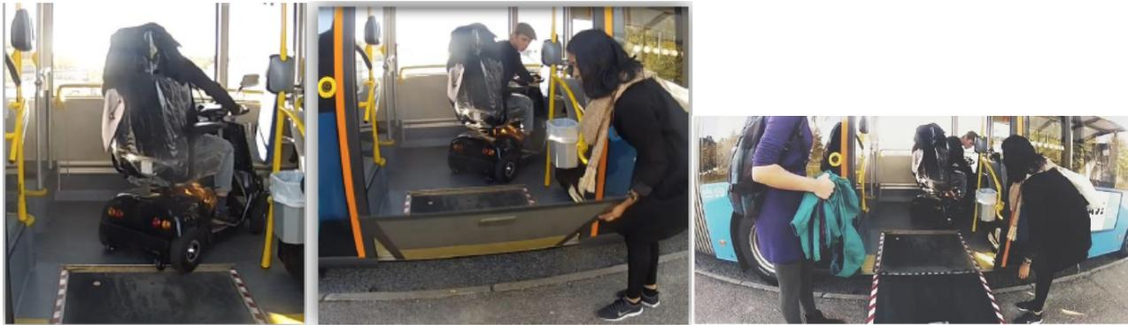
Figure 3 Student project in Gothenburg city testing how busses are adapted for wheel-chairs. The ramp needs to be folded manually and there is limited space for the wheel-chair inside the bus. The wheel-chair driver needs to have an assistant or get help from the driver. The loading/un-loading procedure affects the time schedule of the bus.
