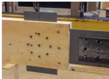
Figure 1. Hierarchically organized experimental program from component tests up to multi-dowel connections.
