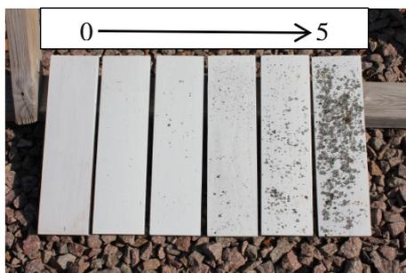
**Fig. 1: Grades of defects / discoloration according to standard ISO 4628-1:2004. Left panel grade = 0, Right panel grade = 5.**
