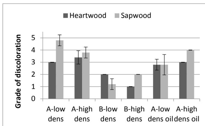
**Fig. 2: Grade of discoloration with standard deviation illustrated as error bars. Sample combinations: A=alkyd, B=acrylate, high density spruce, low density spruce and oil impregnation.**
