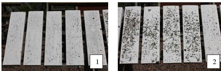
**Fig. 3: Discoloration of Spruce panels coated with an alkyd system (A), low density and no impregnation oil, picture 1=heartwood, picture 2=sapwood.**
