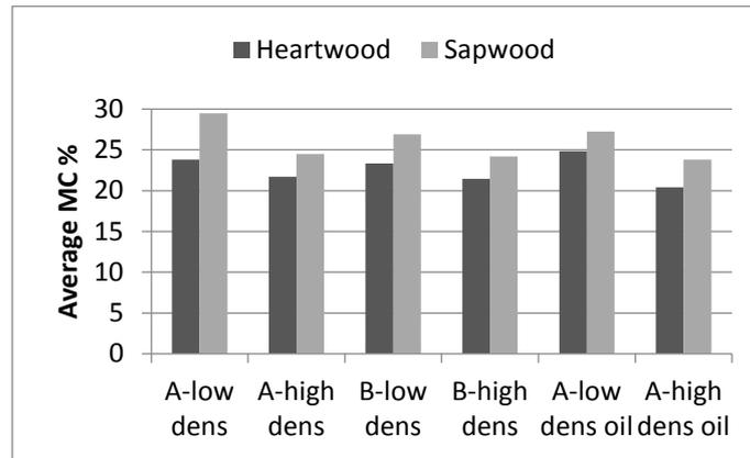
**Fig. 4: Average moisture content. Sample combinations: A=alkyd, B=acrylate, high density spruce, low density spruce and oil impregnation.**
