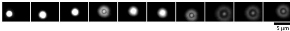
Figure 1. Brownian motion of a latex particle, 2\mu\text{m} in diameter; the time between images is 4\text{ s} ; the movement is in 3-dimensions. Panel 4 and 7-10 show that the bead does not remain in the same focal plane. Picture was taken from [23].
