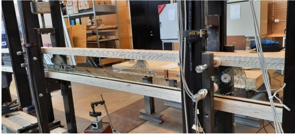
Figure 12: Crack development in the glass web near the load application points, located in the shear-dominated region between the supports and the point loads.
