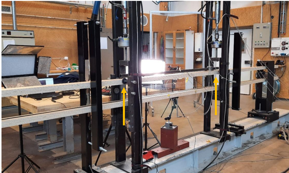
Figure 9: Load test machine used for four-point bending tests. The yellow arrows indicate the locations of the two symmetrically applied point loads on the beam.
