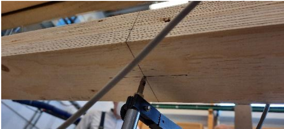
Figure 11: Setup of displacement sensor for global displacement measurement (bottom of beam).
