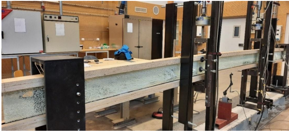
Figure 22: Beams standing after failure of double-layer heat-strengthened glass beams.
