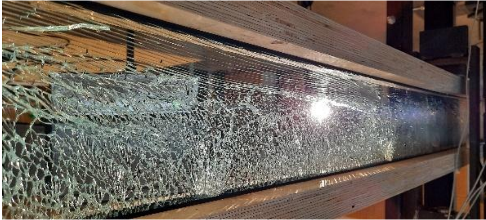
Figure 17: Crack formation in the tested beam showing different perspectives of the same specimen.
