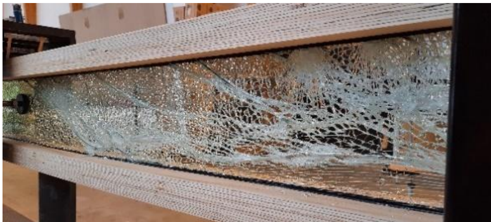
Figure 16: Crack formation in the tested beam.
