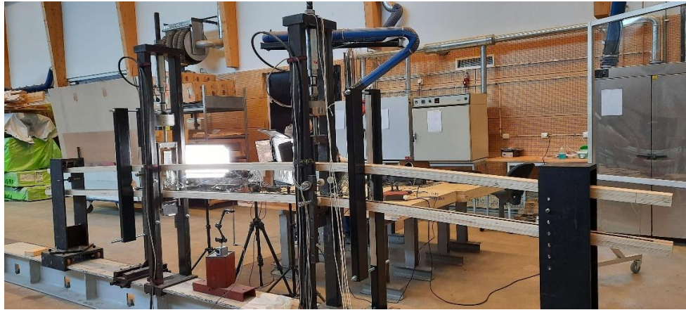
Figure 13: Overall view of the beam after failure showing the final crack distribution and the beam configuration at failure.
