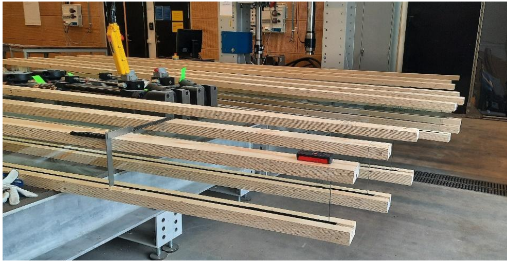
Figure 6: The nine tested composite timber-glass I-shaped beam specimens.
